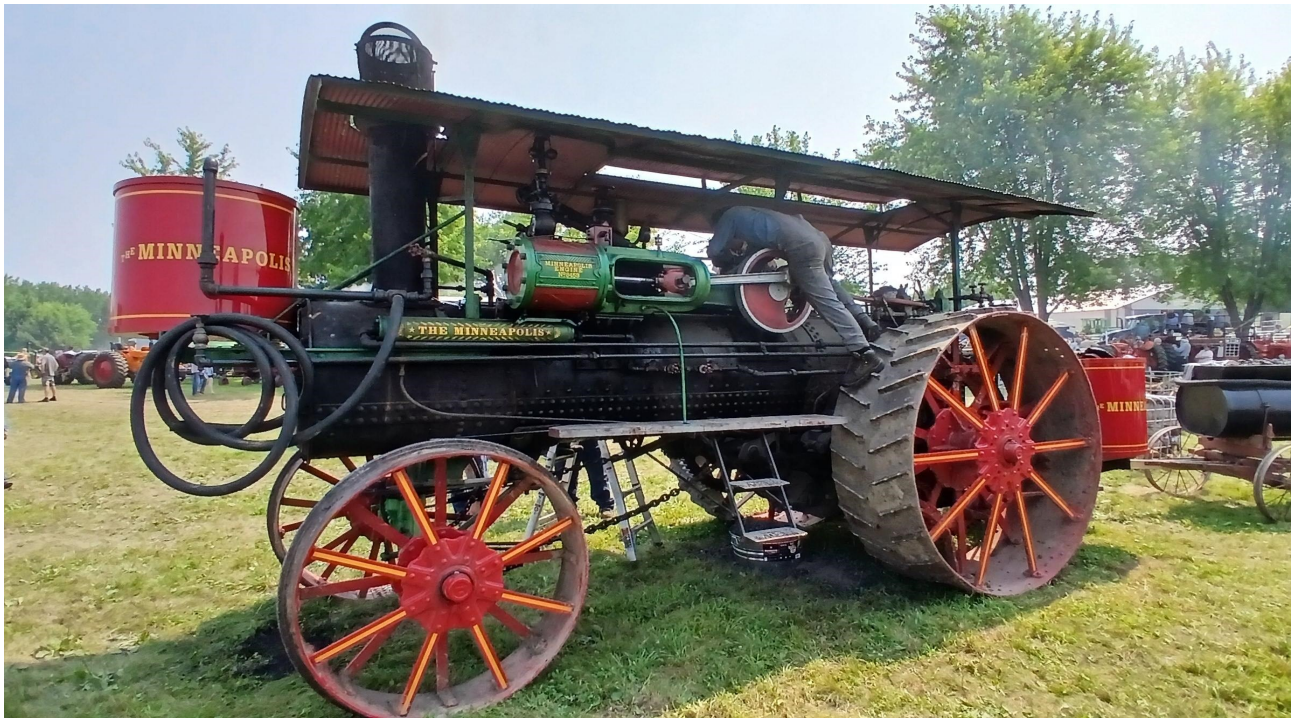
Before gasoline and kerosene/Oil tractors, heavy duty work on some farms was done by steam engines. This 1920 20 H.P. Minneapolis 8453 Steam engine tractor, was used for dray service on heavy loads, field work as plowing, and belt power to run saw mills, threshing machines and the like. Photo Rob Bowe
