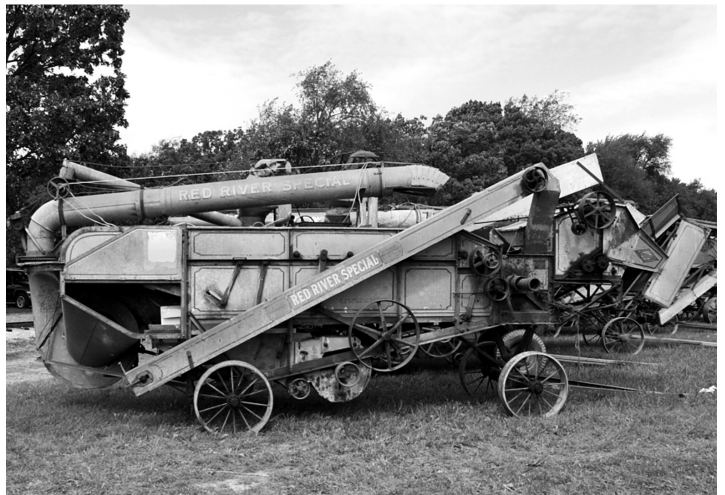
"Red River Special" Threshing machine, made by Oliver Hart-Parr Co. of Charles City, Iowa
